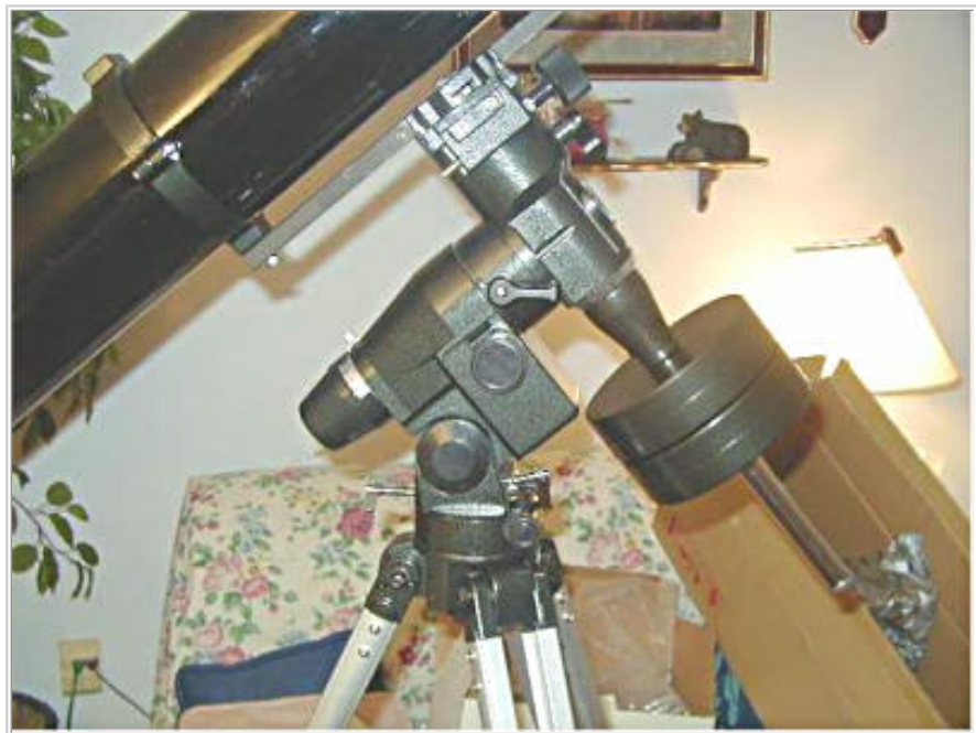
"New" CG-5 with ball bearings. Note the tapered RA housing.
